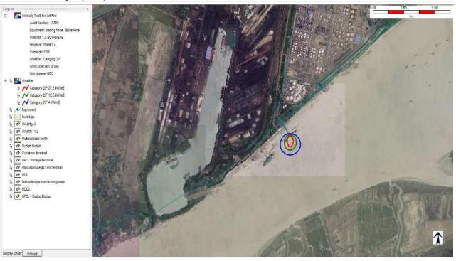
10. Pool fire from Full Bore Rupture of **Butadiene** unloading hose with wind speed 2 m/s and F stability class at Oil Jetty-I (OJ-I).
