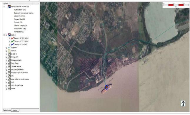
24. **Pool Fire** from Full Bore Rupture of **Xylene** unloading hose with wind speed **2** m/s and **F** stability class at Berth 2.
