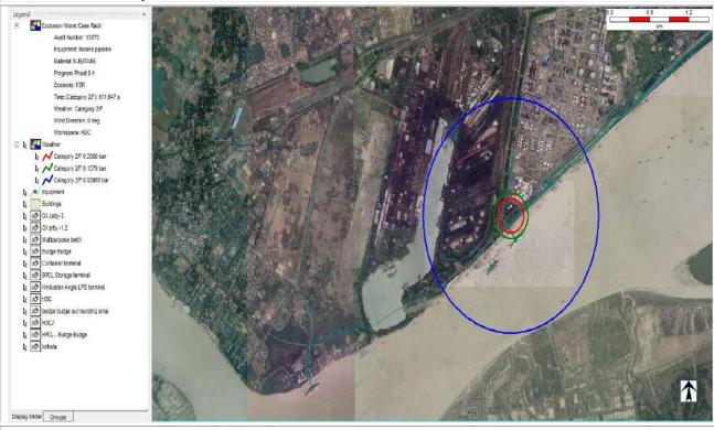
32. Toxic Dispersion from Full Bore Rupture of Ammonia pipeline from Oil jetty-I with wind speed 2 m/s and F stability class.
