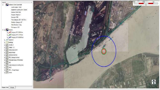
18. Jet fire from Full bore rupture of **Propane** unloading arm with wind speed **2** m/s and **F** stability class at Oil Jetty-III (OJ-III).
