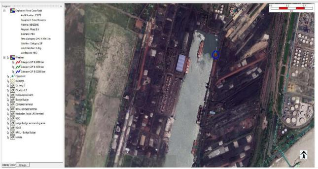
26. Jet fire from Full Bore Rupture of **Propane** pipeline from Oil jetty-I with wind speed **2** m/s and **F** stability class.
