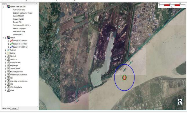
16. **Pool Fire** from Full Bore Rupture of **Butane** unloading arm with wind speed **2** m/s and **F stability** class at Oil Jetty-II (OJ-II).
