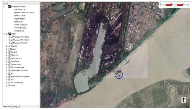
14. Flash Fire from Full Bore Rupture of Propane unloading arm with wind speed 2 m/s and F stability class at Oil Jetty-II (OJ-II).
